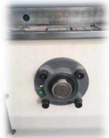
An automated lubrication pump for the feed track is included – simple and effective.
