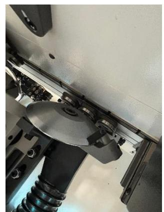
The radius scrapers are followed by a second set of flat glue scrapers.
