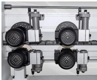
extra heavy (40 and 50mm diameter!) mounts that deliver a heavy duty vibration free finish.
