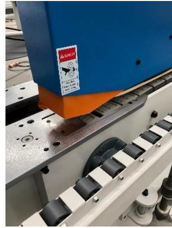
Electronic monitoring eliminates any chance of the gap between panels being too short. The timing is varied automatically dependent on what working stations you have activated. This is better than a 'red light/ green light' system which relies on the operator obeying the light!
