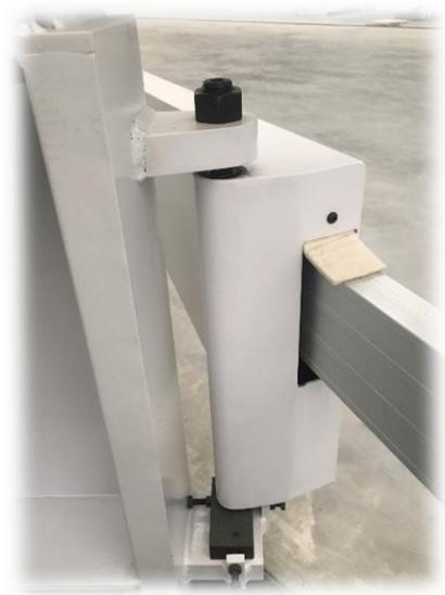
The crosscut fence is 90 x 80mm and strongly mounted for precise 90-degree cuts. All settings are clear via large recessed steel scales
