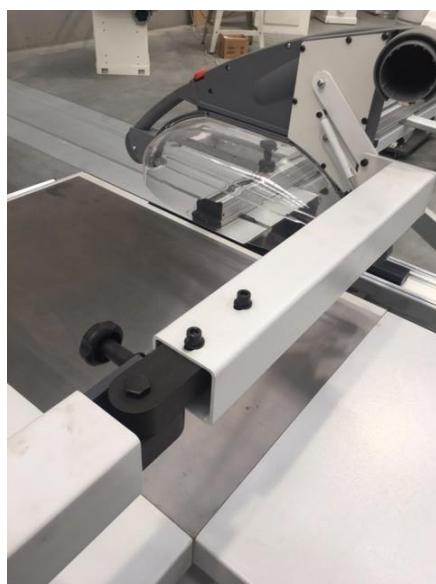
A strong pivot joint allows the guard to swing clear when required.
