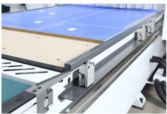
Table bed is constructed from 12-20mm thick steel
