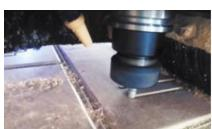
Additional blowing of the processing zone ensures effective removal of chips from the cutting zone, which significantly affects the
