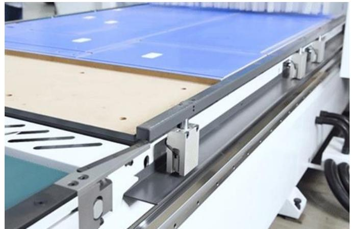
***Table bed is constructed from 12- 20mm thick steel***
