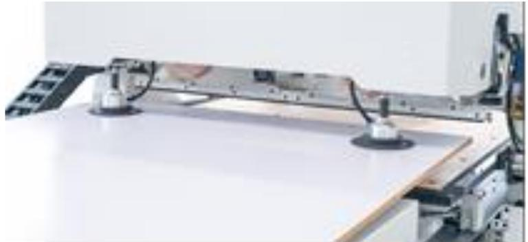
A new sheet is loaded at the same time as the completed nest is pushed off:
