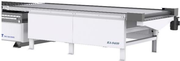
*You or we can supply a simple static outfeed sorting table— or KDT have a clever driven outfeed table option with extraction and light sensor control – perfect for JIT labelling*
