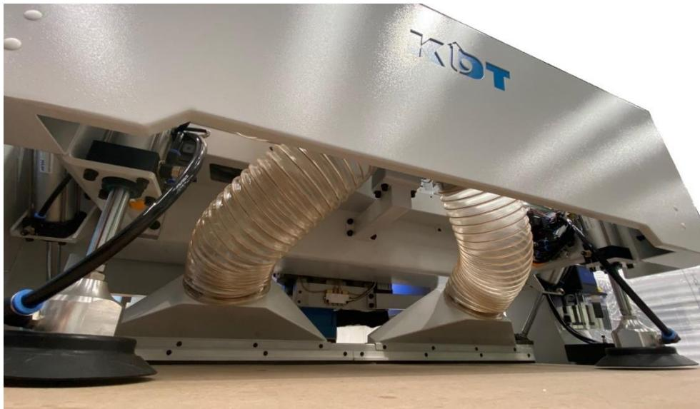
A smart unloading pusher with built in extraction pushes the completed nest to a sorting table. You can immediately load a new panel and commence your next nest effectively doubling your output.
