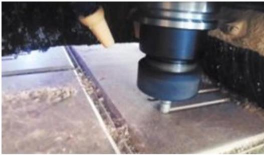
Additional blowing of the processing zone ensures effective removal of chips from the cutting quality of processing and tool life.
