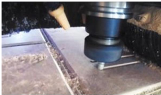
Additional blowing of the processing zone ensures effective removal of chips from the cutting zone, which significantly affects the quality of processing and tool life.
