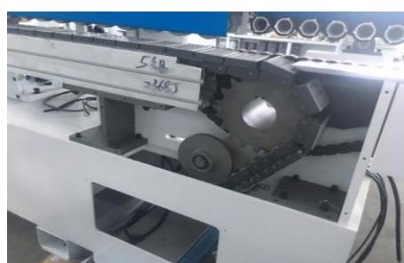
The feed track runs on square and round guides guarantee no sideways movement or tilt under load. Cast bearing housings and heavy chain feed ensure long service life
