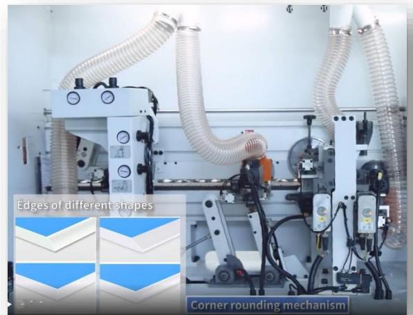
Programmed from the touch screen the two-motor unit delivers precise finishes even on post formed and finger pull – and fantastic results on square edge panels
