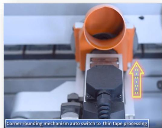
Reset from thin to thick tape – automatically from the touchscreen or within a Program
