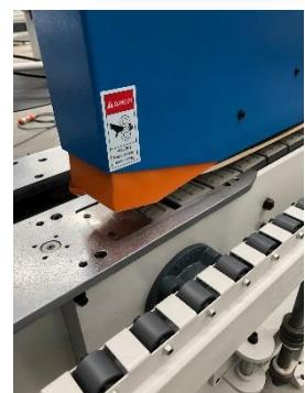
To eliminate any chance of the gap between panels being too short there is a pneumatic pin that prevents a second panel entering too soon. The timing is varied automatically dependent on what working stations you have activated.
