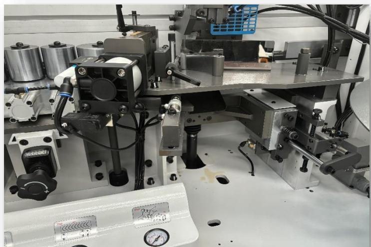
The hard chromed 100mm first driven roller does the initial application. Rollers 2 and 3 are tapered – 1 applying extra pressure at the top edge and the other at the bottom to close the glue line for a magic result. Roller 4 is the final guarantee of the perfect tight edge your customers will love. The pressure rollers are adjusted all together / digitally for different tape thickness
