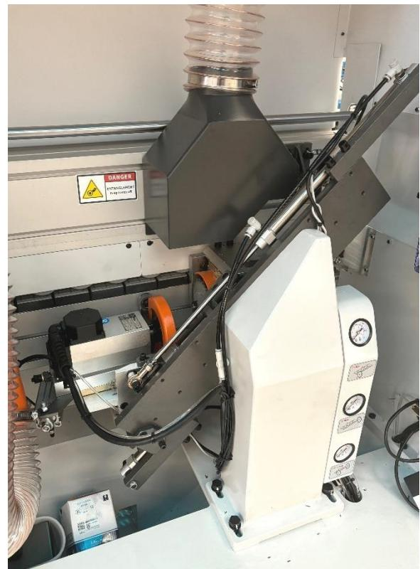
Independent 12,000 rpm inverter controlled saw motors ensure clean, effortless trimming of your toughest tapes.
