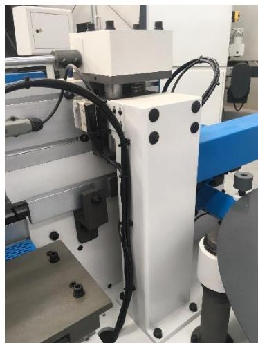
The overhead feed rollers are mounted in a heavily ribbed aluminium top beam 170mm x 80mm.
