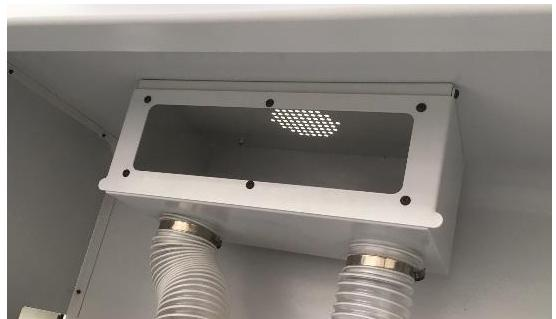
The scrapings are exhausted into an easily accessed separation/ collection box, so they do not foul your dust extractors fan / filters
