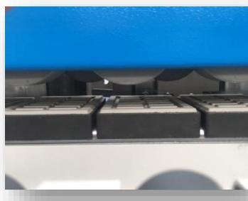
Overhead feed rollers are mounted in a heavily ribbed aluminium top beam 170mm x 80mm. Oversize Beam supports ensure alignment without flexing under load. A clever tensioning system guarantees parallel alignment.
