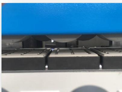
Overhead feed rollers are mounted in a heavily ribbed aluminium top beam 170mm x 80mm. Oversize Beam supports ensure alignment without flexing under load. A clever tensioning system guarantees parallel alignment.
