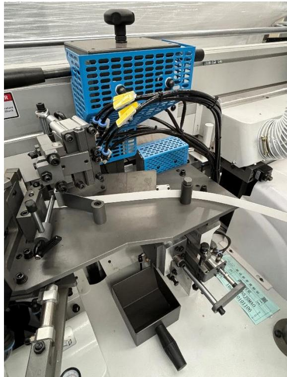
The entire tank simply unplugs thanks to quick unclick electrical and pneumatic connectors and is then easily removed in around 2 minutes. This is a clean and fuss free system with easy top access to replenish and keep an eye on glue levels. You can also stop glue feed to the roller at the flick of a switch,
