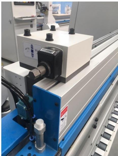
The feed track must ensure panels stay perfectly aligned through the machining groups. Overhead feed rollers are mounted in a heavily ribbed aluminium top beam 170mm x 80mm. Oversize Beam supports ensure alignment without flexing under load. A clever tensioning system guarantees parallel alignment.
