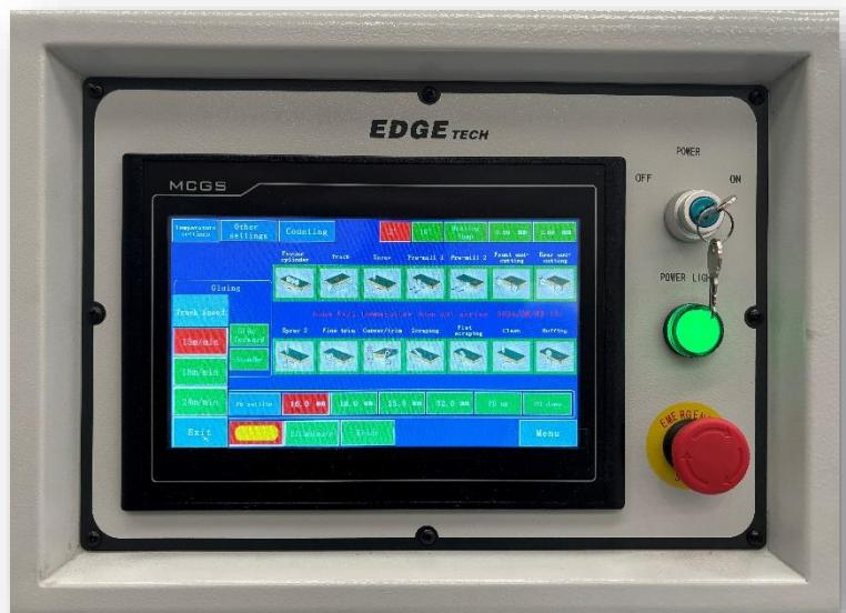
Reset your trimming stations from the touchscreen with KDT's simple digital pneumatic system
