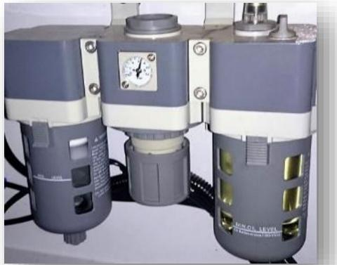
**Pneumatics:** Water separator and automatic lubrication of pneumatics.
