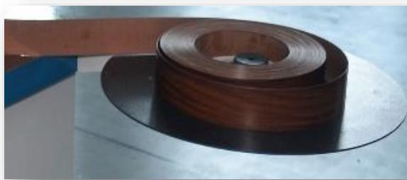
Large 800mm diameter and heavy duty rotary tape coil tray
