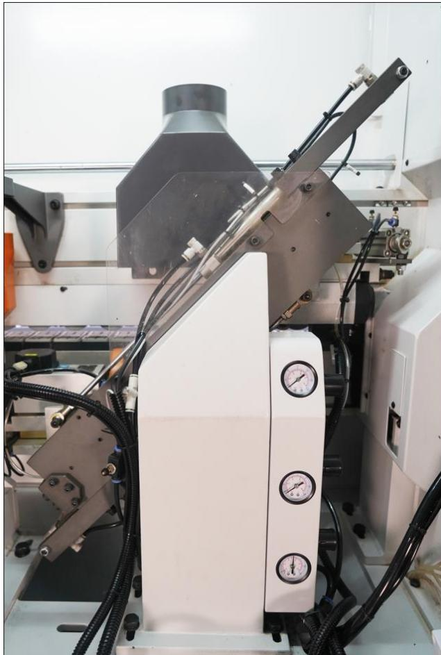
The saws are mounted on a cast iron base and single high precision THK guide for perfect alignment
