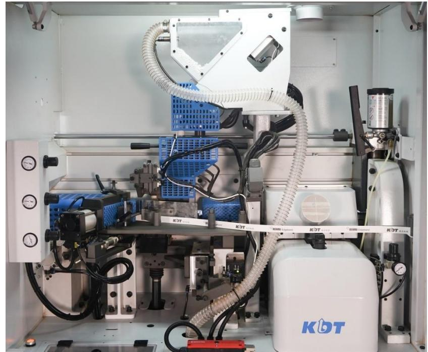
Unique ejection function for auto cleaning of the glue roller
