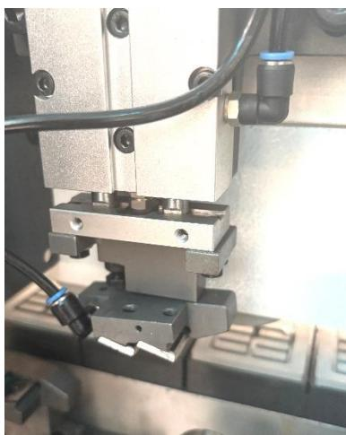
The scraping unit is equipped with two carbide radius knives, which after milling the edge remove a thin layer from the milled part of the edge and remove the wave, as a result we get a smooth processed surface. The scraping unit is equipped with a mechanism for separating chips from the workpiece after scraping.
