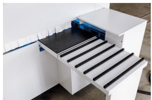
The minimum workpiece size is 70x35 mm, which allows for the addition of small-sized parts.
