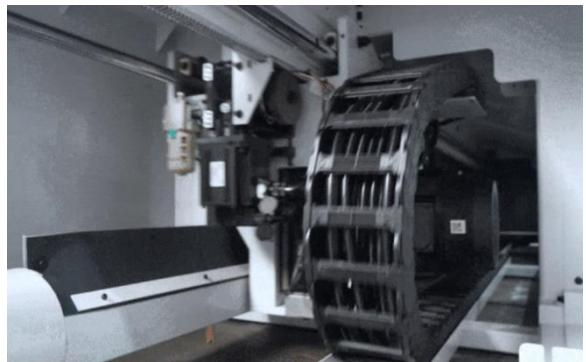
Heat treated precision rack and large diameter pinion drive for the saw carriage.
