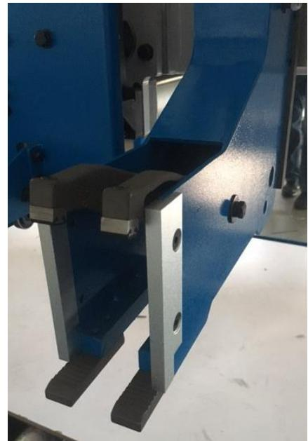
Heavy duty cast aluminium gripper construction: years of trouble - free service.
